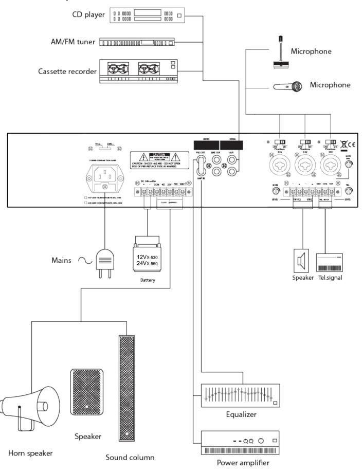
**EXPAND THE INPUTS** – It is possible to expand the inputs of the X-530/560 using the V-RVC-PRO (remote mic/line mixer) and the X-Music (in-wall iPod Smart Phone dock). The V-RVC-PRO is capable of expanding the X-530/560 inputs to a maximum of 9 over Cat5/6 cable. See the diagram below.
