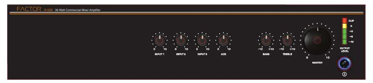
**Bass -** The bass control is a shelving type equalizer that boosts or cuts bass frequencies at 100Hz +/- 12 dB. The center "0" position does not affect the signal. Equalizers should be used sparingly. Too much boost can cause feedback when using microphones.
