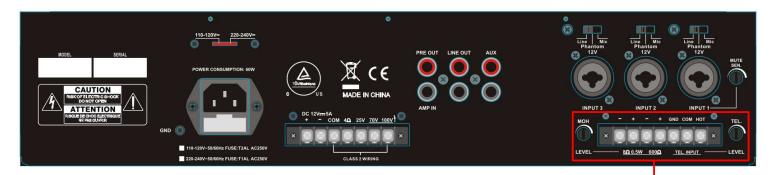
**TEL INPUT** – This is a balanced audio input that is designed to accept signals from an analog telephone output. Due to the varied output levels from different telephone systems we have provided a level control that allows precise level adjustments.
