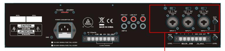
**Mute SEN –** The Mute SEN adjusts the level of override. Fully counter clockwise reduces the sensitivity where more of the background music would be heard. A high input level would be necessary to trigger the override circuit. Fully clockwise increases the sensitivity where a low input level would trigger the override circuit and the background music would be completely muted. Adjust this control to achieve your desired results.
