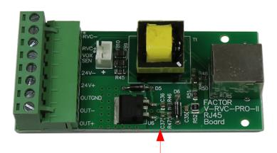
**New!** Ultra low-noise circuits & transformer isolated balanced outputs for Cat6 runs of over 1000'
